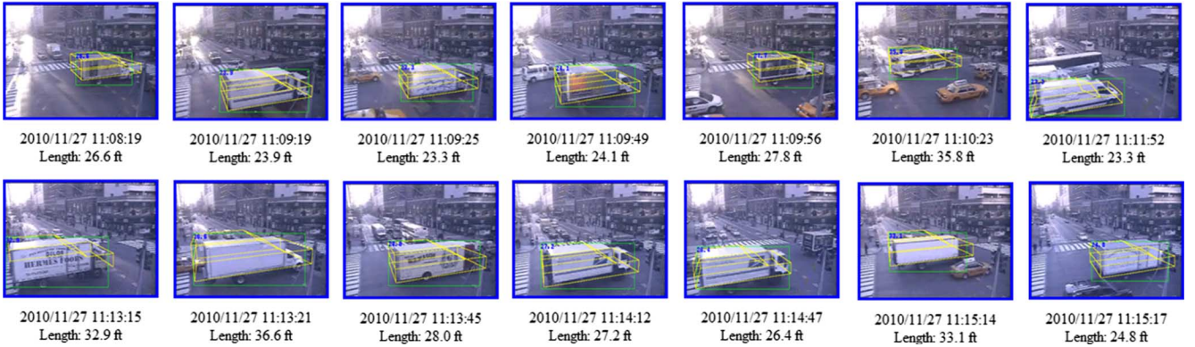
Fig. 19. Example of a search for large vehicles (larger than 18 ft.). Our vehicle detection method provides precise bounding boxes for multiple types of vehicles. Real vehicle dimensions in world coordinates are then obtained through a calibration and 3-D model fitting process.
