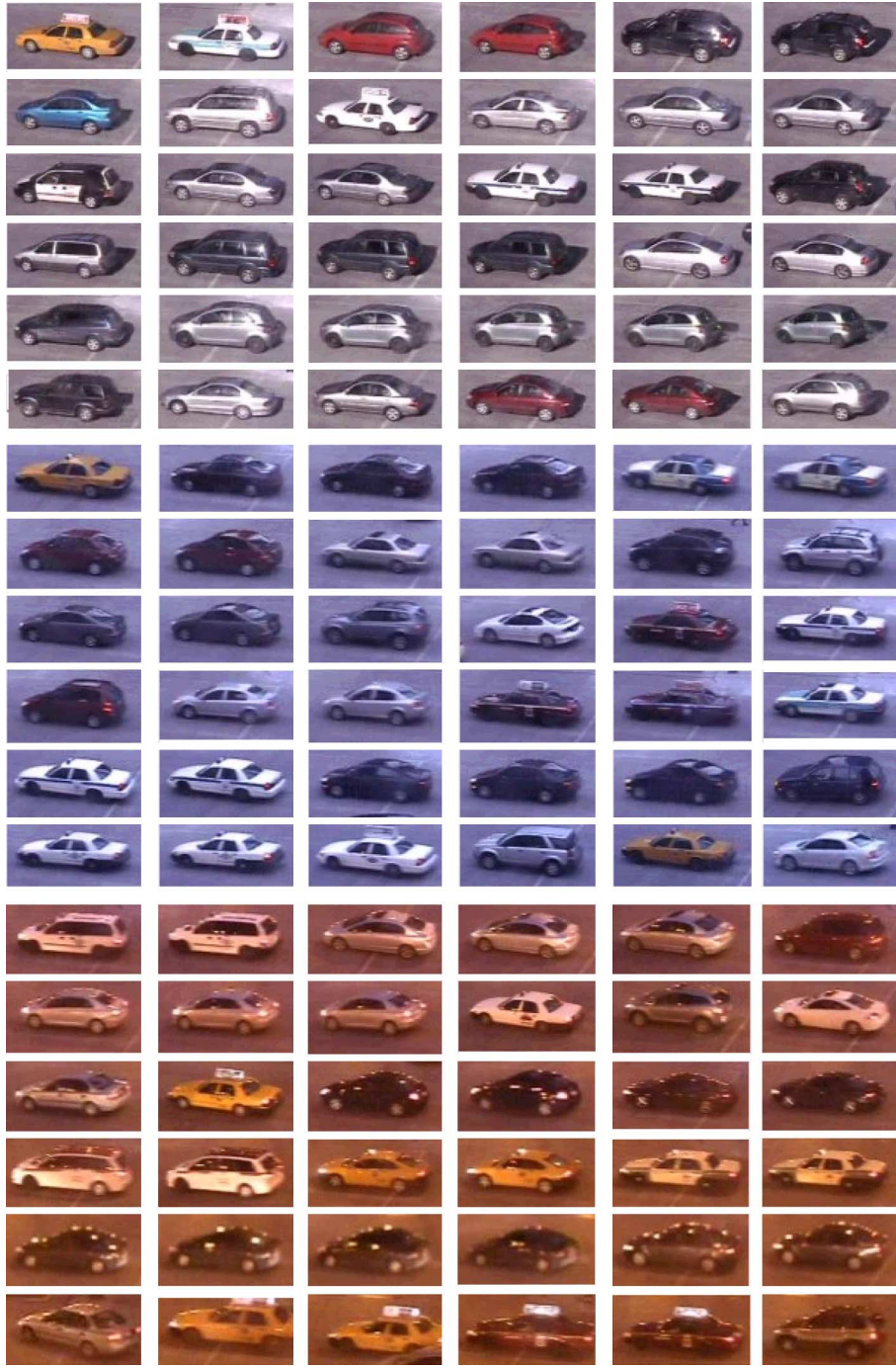
Fig. 4. Automatically collected data for a specific vehicle pose in different time periods. See http://rogerioferis.com/IEEEMultimedia/SideView-1.wmv for a video demo. For this specific sequence, we are able to capture more than a thousand cars without false alarms.
