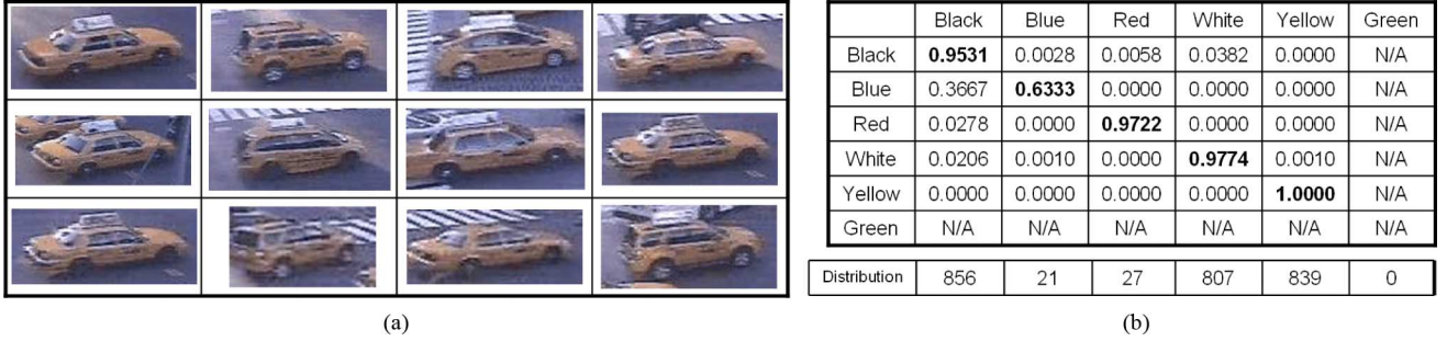
Fig. 18. Color retrieval results. (a) Example results for a yellow car search. Note that for this particular scene, all taxi cabs have yellow color. (b) Quantitative results—confusion matrix and color distribution for the captured vehicles.
