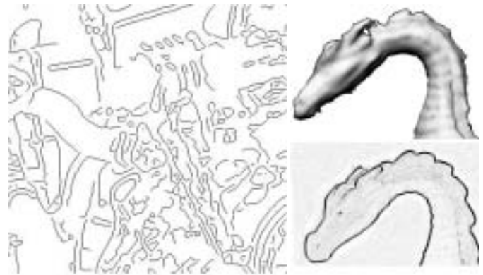
Figure 17: (Left) Intensity edge detection (Canny) for engine of Figure 1(a). (Right Top) Depth map from 3Q scanner, notice the jagged depth edges on the neck. (Right Bottom) Depth edge confidence map using our technique.
