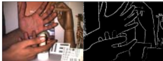
Figure 14: (Left) A frame from a video sequence, shadows due to left flash. (Right) Detected depth edges merged from neighboring frames.
