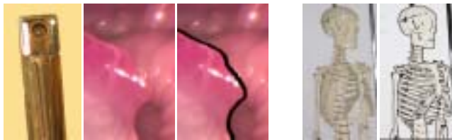
Figure 16: (Left) Enhanced endoscope, with only left lights turned on; input image and depth edge superimposed image. (Right) Skeleton and depth edge superimposed image.
