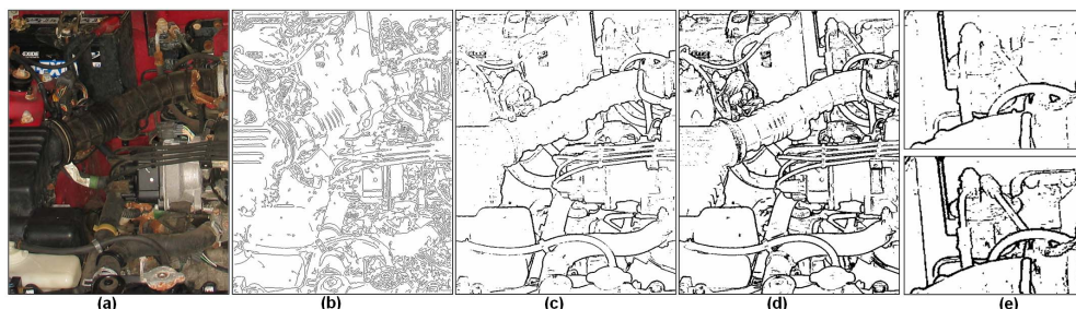
Figure 8: (a) Complex scene with different amounts of changes in depth. (b) Canny edge detection. (c) Depth edges computed with one single camera-flash baseline. (d) Depth Edges computed with our multibaseline approach. (e) Part of the engine zoomed in to compare single-baseline depth edges (top) with our multibaseline method (bottom).
