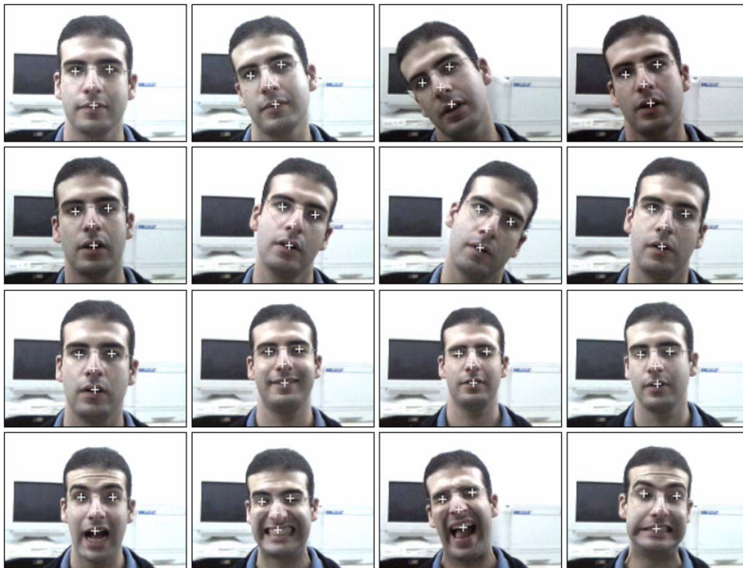
Fig. 4. Sample frames of our wavelet subspace tracking. Note that the tracking method is robust to facial expressions variations as well as affine deformations of the face image.
