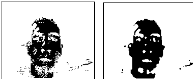
Fig. 6. Thresholding and morphological closing followed by median filtering
