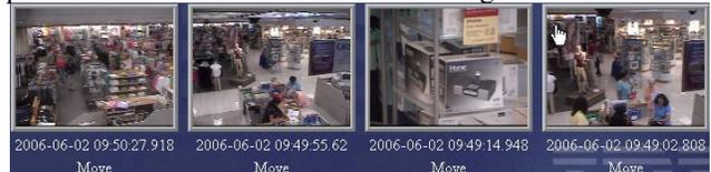
Figure 3: Database alerts generated by moving a camera
